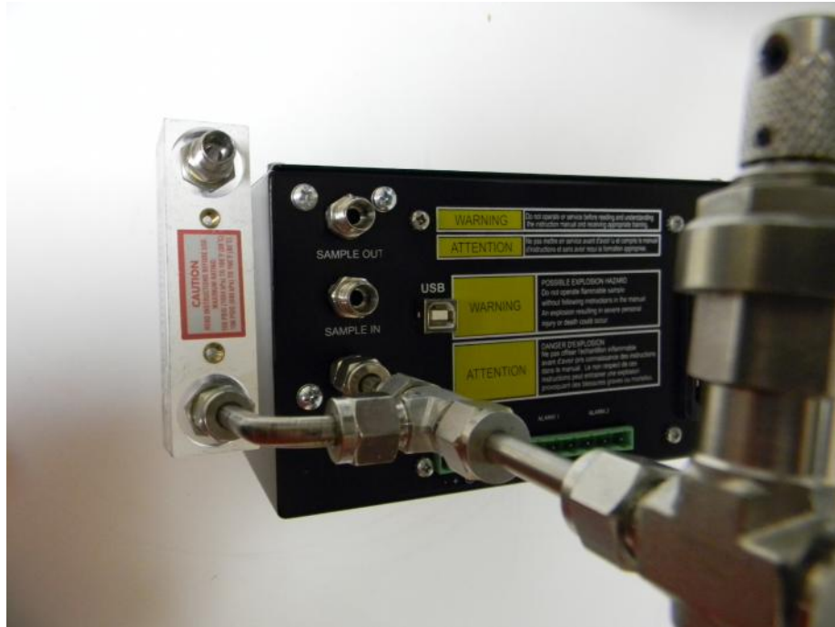
Figure 8 Span gas bypass connection – back view.
